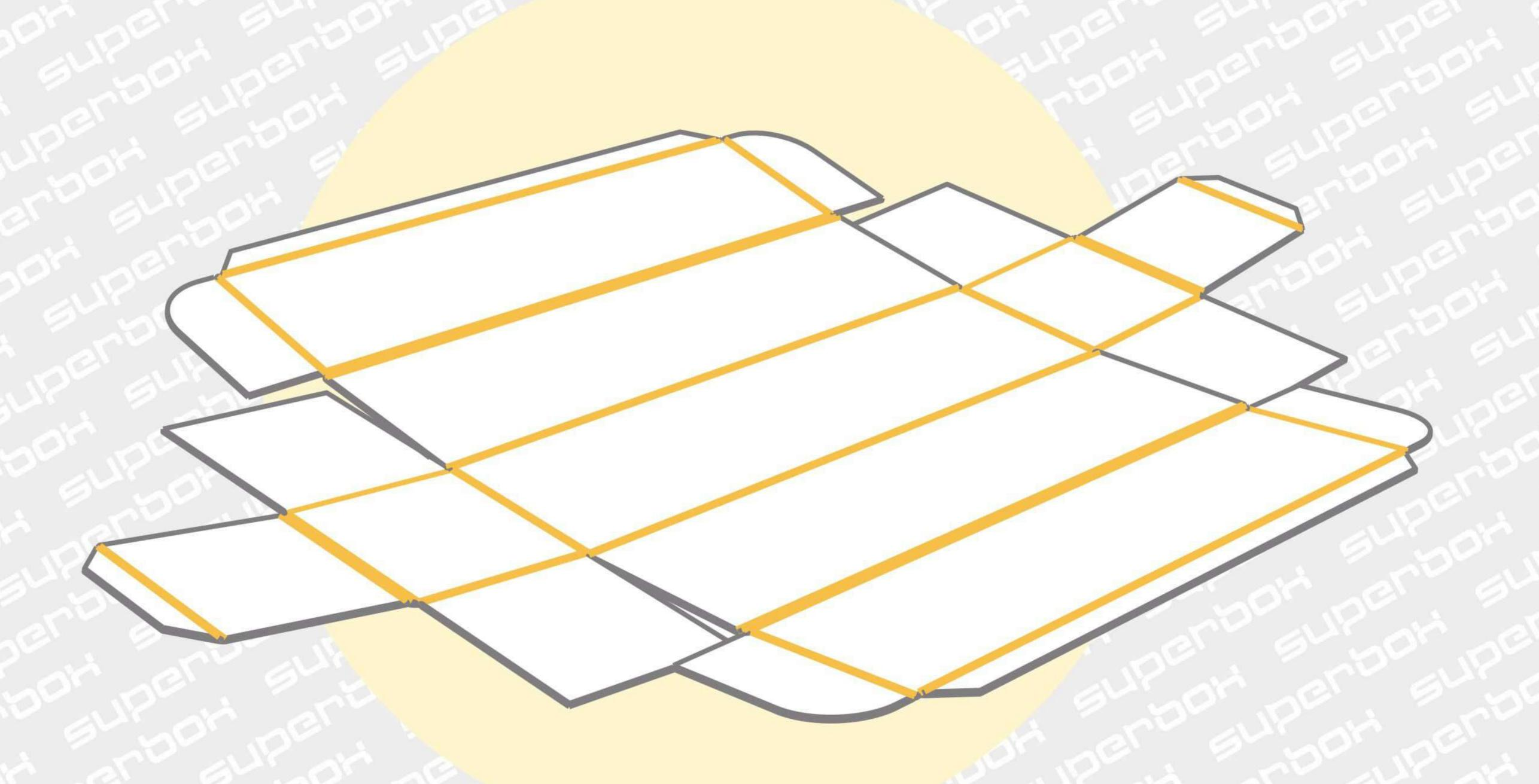
Position these side walls and fold in the inner flaps. \* Start folding from the walls with the flaps closer to the plane of the lid.
