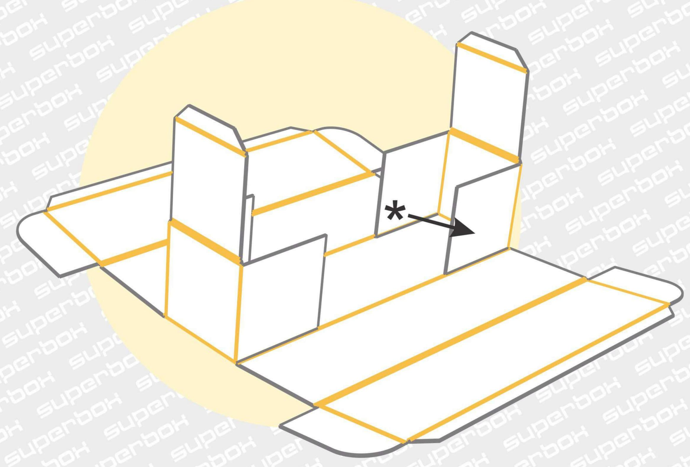
Fold out the small flaps and the narrow curb of the remaining two walls to the opposite side and fold these walls over to enclose the flaps described in step 2. \* Make sure that the two bending lines of these walls are aligned.
