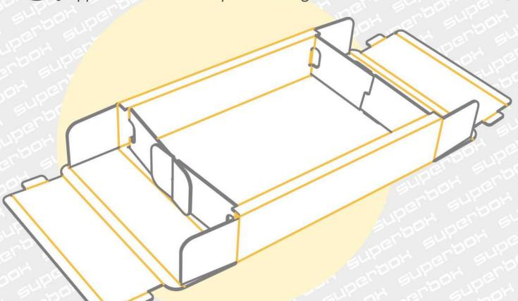
Fold the small flaps over the already folded walls and fold the remaining side walls around the folded ears and small flaps. \* fold the small fixating latches while bending the wall. They must fit into the holes on the plane of the locking earflaps.
